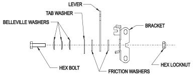
FIGURE 13 THROTTLE TENSION
